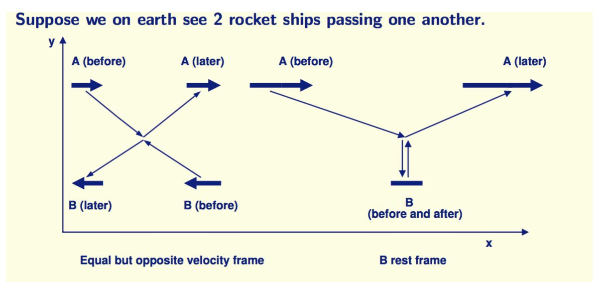
Figure 11: Depiction of two rockets passing one another: a) in equal but opposite velocity frame, each having velocity of magnitude v'; b) in B rest frame, where velocity of A appears to be v.
