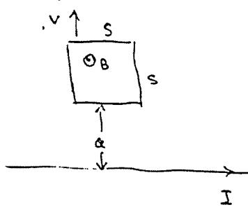
$$\text{Flux} = \int \vec{B} \cdot d\vec{a} = s \int_a^{a+s} B(r) dr = s \int_a^{a+s} \frac{\mu_0 I}{2\pi r} dr = \frac{\mu_0 I s}{2\pi} \ln \frac{a+s}{a}$$
